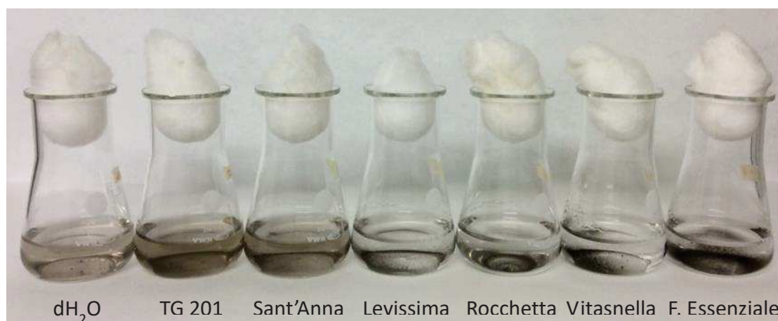
Figure 1. Visual inspection of GO dispersions (20 \text{mg L}^{-1} ) in \text{dH}_2\text{O} , TG 201 medium, Sant'Anna, Levissima, Rocchetta, Vitasnella and Fonte Essenziale, after 72 h.
