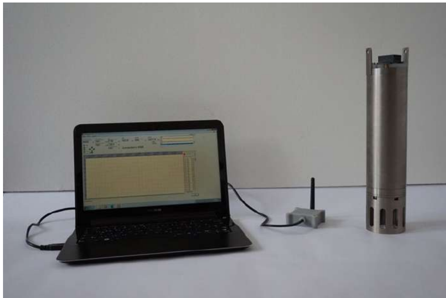
Figure 1: Measuring system with multiparameter probe, wireless transmission and evaluation software
