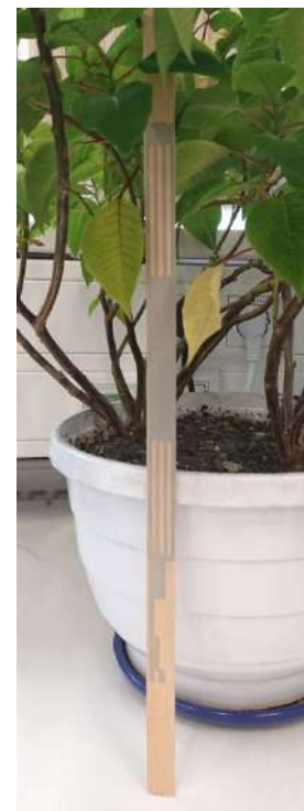
b) Printed antenna on wood carrier
