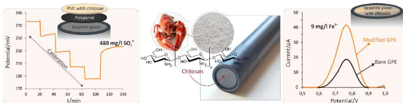
Figure 1: Modifications of graphite paste electrodes with chitosan for the potentiometric measurements of sulfate ions (left) and for the voltammetric determination of iron ions (right).
