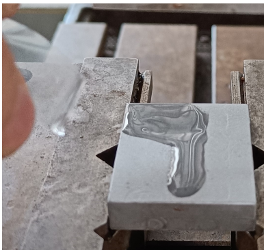
(g) Glue spreading on the steel surface.
