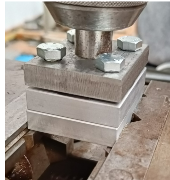
(f) Aligning of the steel plates before gluing.
