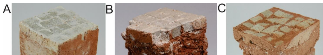
Figure 92 Specimen M17: A) Before degradation process; B) after degradation; C) after restoration process.
