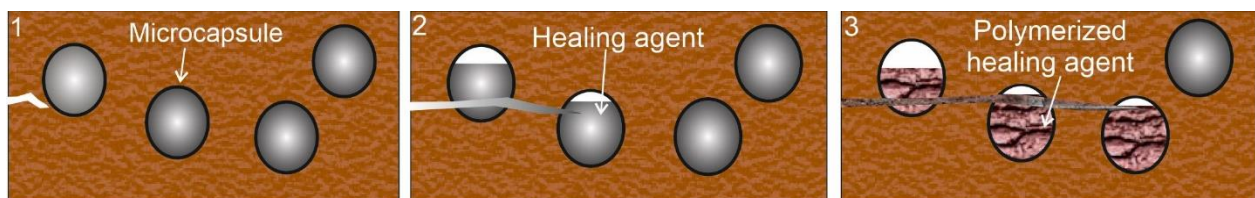
Figure 16 Process of self-repairing thanks to polymeric microcapsule.
