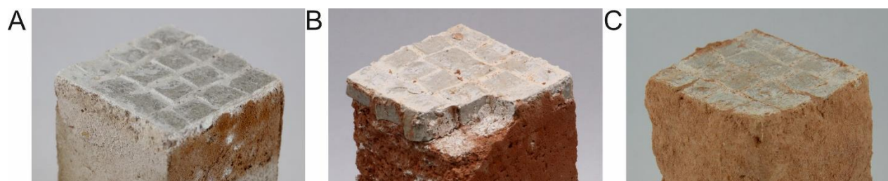
Figure 91 Specimen M26: A) Before degradation process; B) after degradation; C) after restoration process.
