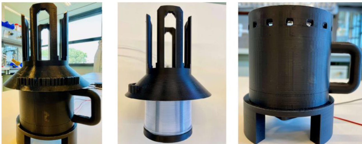
Figure A 24: Overview of the 3D-printed flow reactor. Left: overall reactor; middle: inside of the reactor (flow loop) and holder for the Kessil lamp in the center; right: main body, internally coated with reflective tape. A fan is mounted on the bottom to keep the temperature stable around 30–33 °C.
