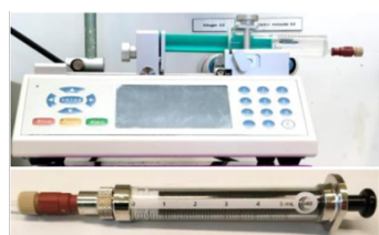
Syringe pump (Chemyx Fusion 200) and Gastight syringe (SGE Luer Lock 5 mL)
