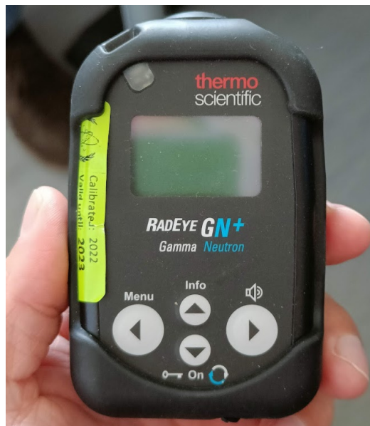
Figure 1.6: ThermoFischer active \gamma/n dosimeter at NSIL, IAEA. This is an example of an embedded system targeting nuclear instrumentation: a self-contained portable device adapted to reliably accomplish a specific task.
