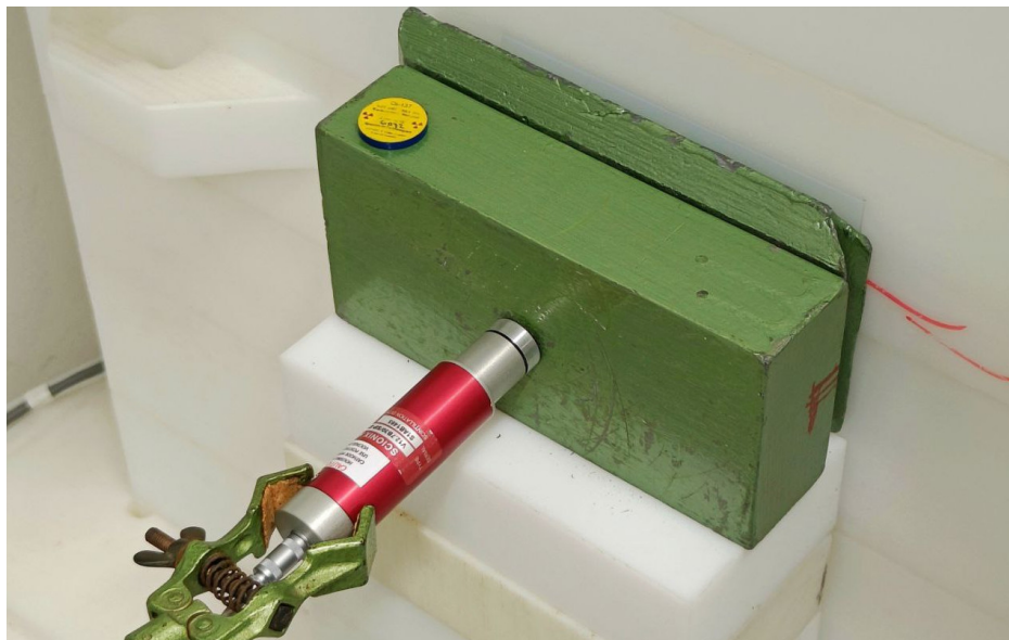
Figure 5.3: Integrated CLYC detector placed at the output window of the DD generator, separated by a lead block to maximize the Cs-137 \gamma counts, used for energy calibration.
