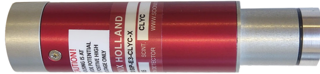
Figure 1.5: Integrated CLYC detector (Scionix V12.7B30/SIP-E3-CLYC-X). It includes a small CLYC scintillator optically coupled to a SiPM array, a temperature-compensated bias supply, and an output preamplifier.
