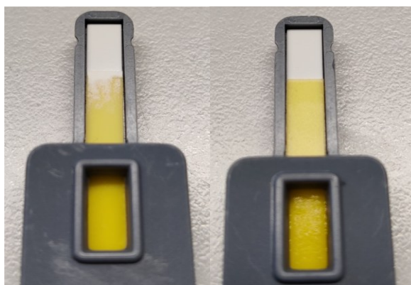
Figure 10. On the left, an example of a non-complete saturation of a test strip. A white jagged zone is clearly visible on the membrane region farthest from the filter. On the right, a complete, normally saturated membrane. Bilirubin-spiked plasma was used for this test, TSB concentration was around 16 mg/dl.
