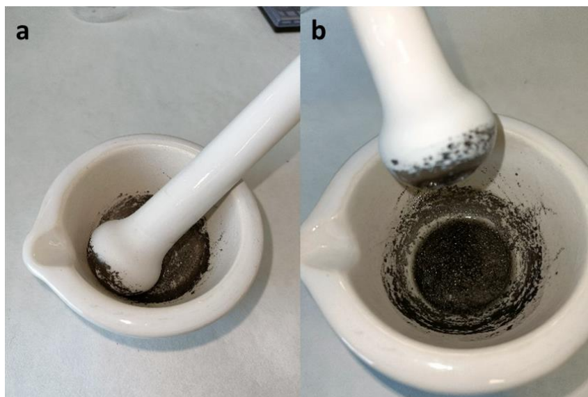
Figure 85 a) Graphite grinding; b) grinding of graphite + Cyrene.
