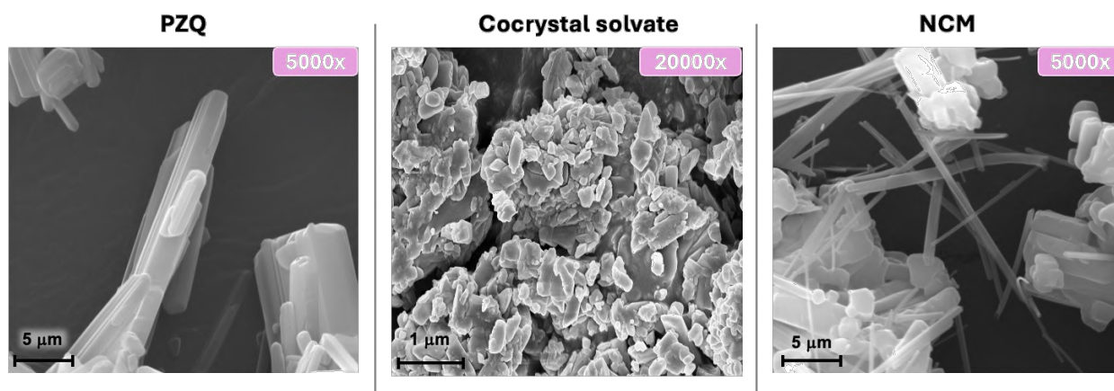
Figure 50. SEM images of (a) PZQ (5000x), (b) PZQ-NCM-AA cocrystal solvate (20000x) and (c) NCM (5000x).
