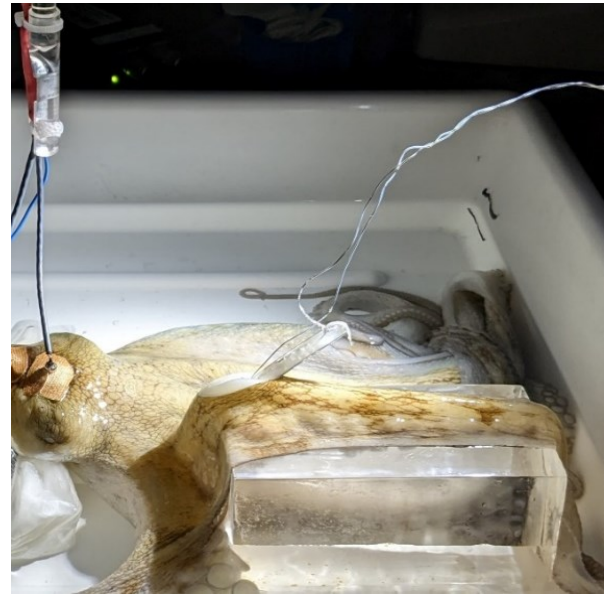
Figure S.3. Silver teflon-coated hook electrode anchored to isolated arm nerve cord during electrophysiological recording.
