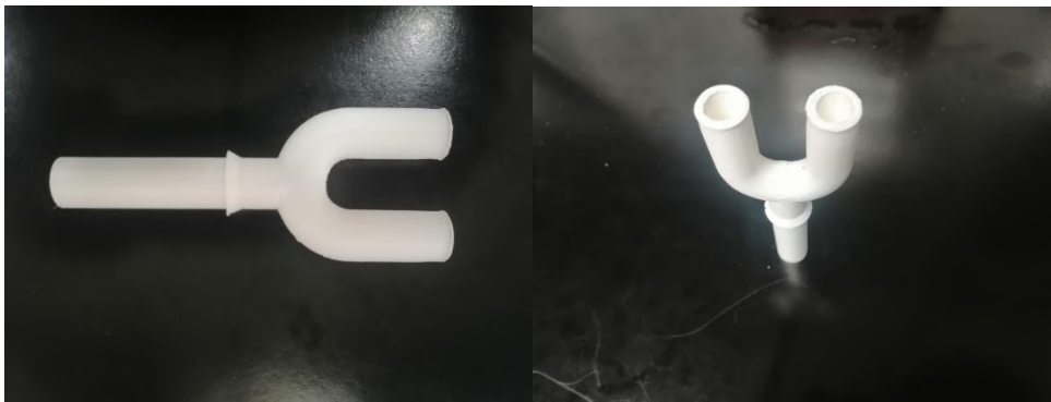
Figure 9. Photographic images of the Y shaped tube sampling port
