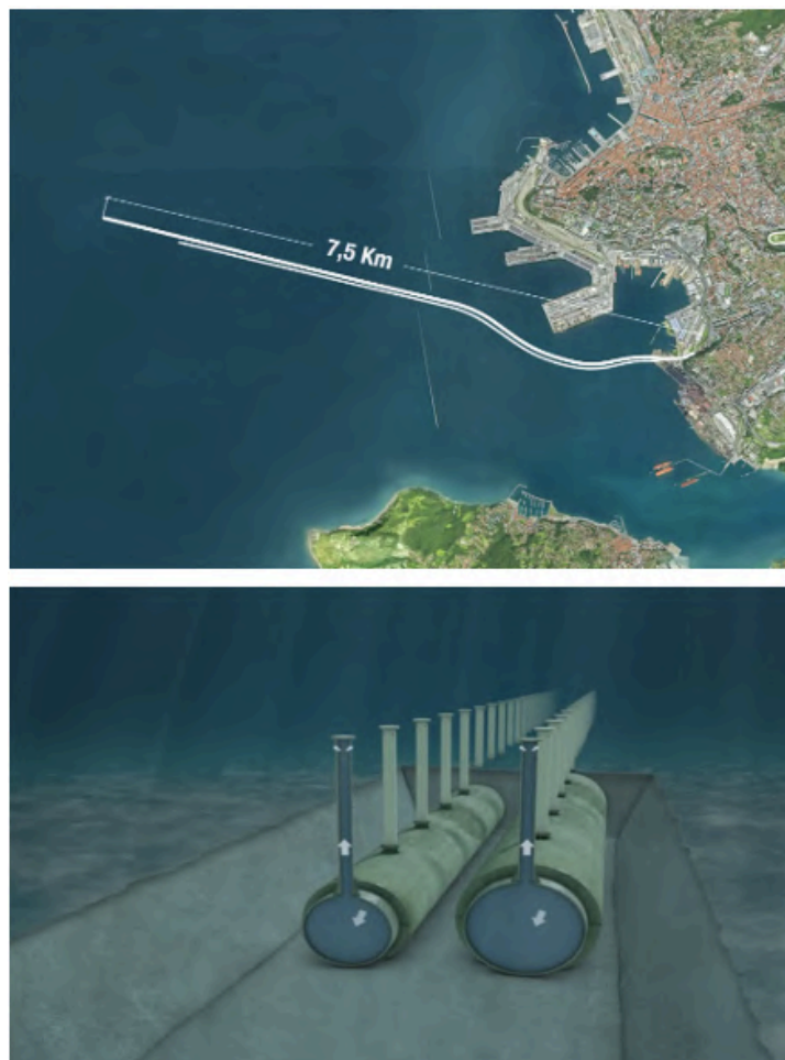
Figure 25. Duct that extends approximately 7 km into the Gulf of Trieste, where releases homogeneously the treated water of the WWTP of Trieste through a system of 600 “towers”.
