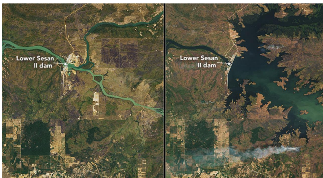
Figure 1.3 - Example of how a large land-consuming hydropower project could affect the landscape, with consequent negative impacts on habitat connectivity. On the left is the landscape before construction of the dam, while on the right is the landscape during the operational phase of the hydropower project. Source: https://earthobservatory.nasa.gov/images/91761/a-new-reservoir-in-cambodia .
