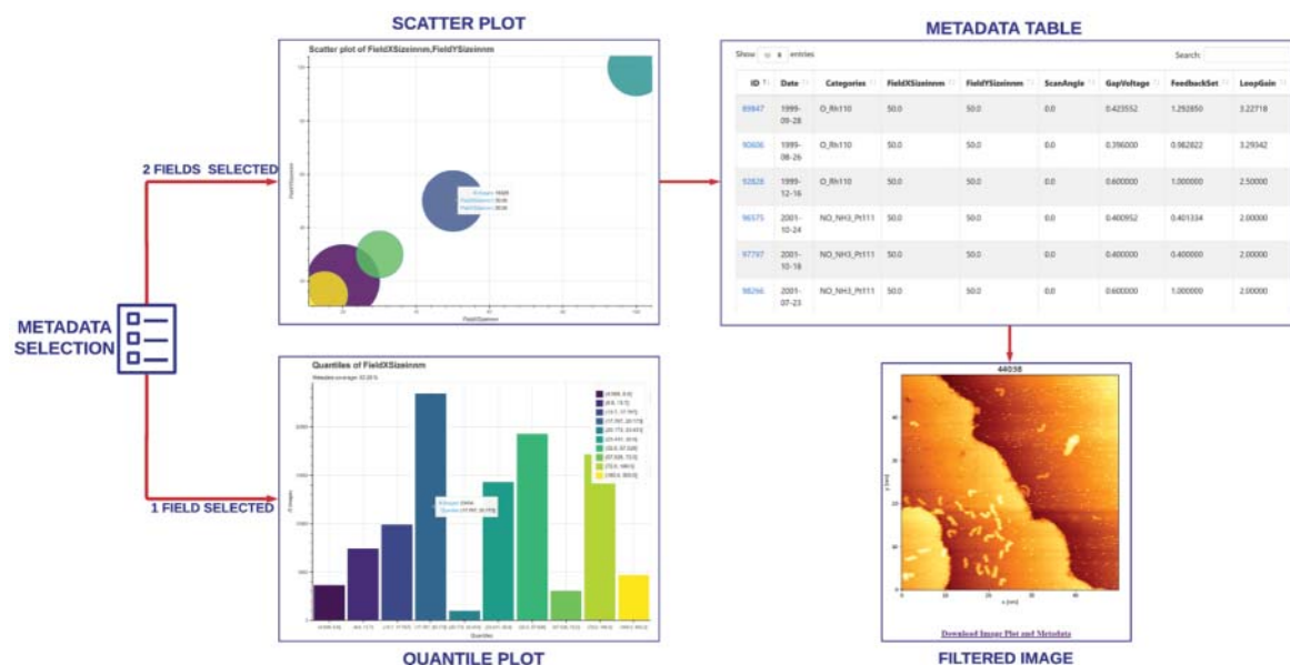
Figure 3. The web service workflow on the TriDAS website. Users select metadata and based on the fields selected, can explore the images metadata through a quantile plot for a single metadata field and a scatter plot that shows the distribution of images between two chosen metadata fields.
