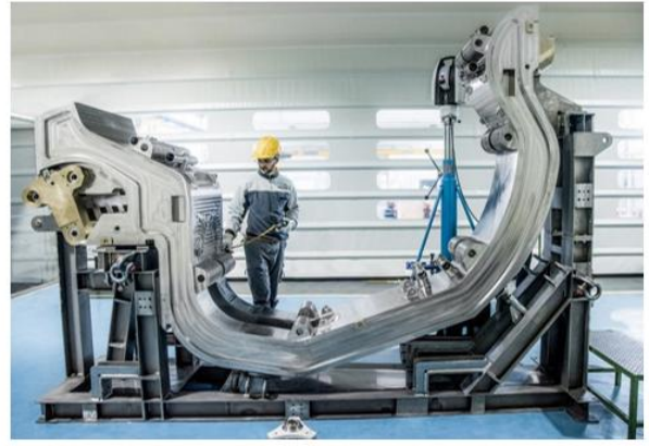
Figure 20 ITER Tungsten Divertor Outer Target (left)-ITER Divertor Cassette Body (right) [31]
