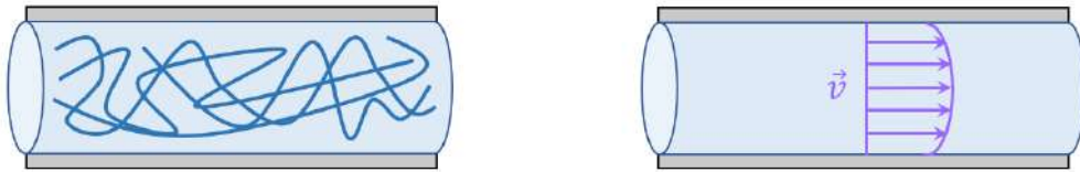
Figure 7.1: Streamlines and velocity profile for turbulent regime flows.
