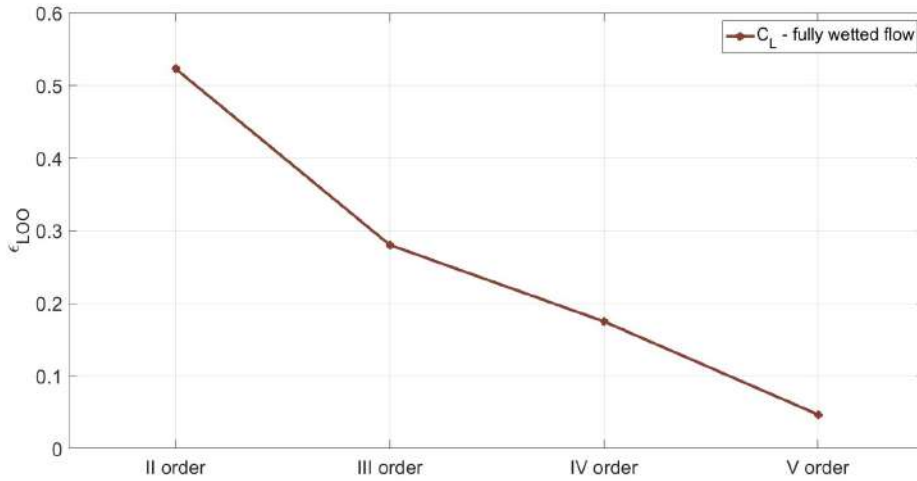
Figure 11.5: Leave-One-Out Cross-validation error trend of the lift coefficient in the fully wetted flow condition - NACA66(MOD).
