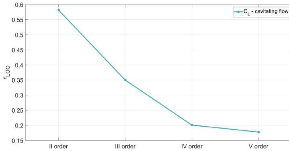
Figure 11.33: Leave-One-Out Cross-validation error trend of the lift coefficient in the cavitating flow condition - NACA66(MOD).
