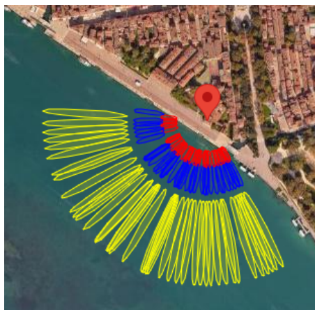
Figure 3.9: Reflection zones for VEN1 station. The colors represent different elevation angles (5° yellow, 10° blue, 15° red). The azimuthal angles from which the useful SNR values come from are between 150° and 280°.
