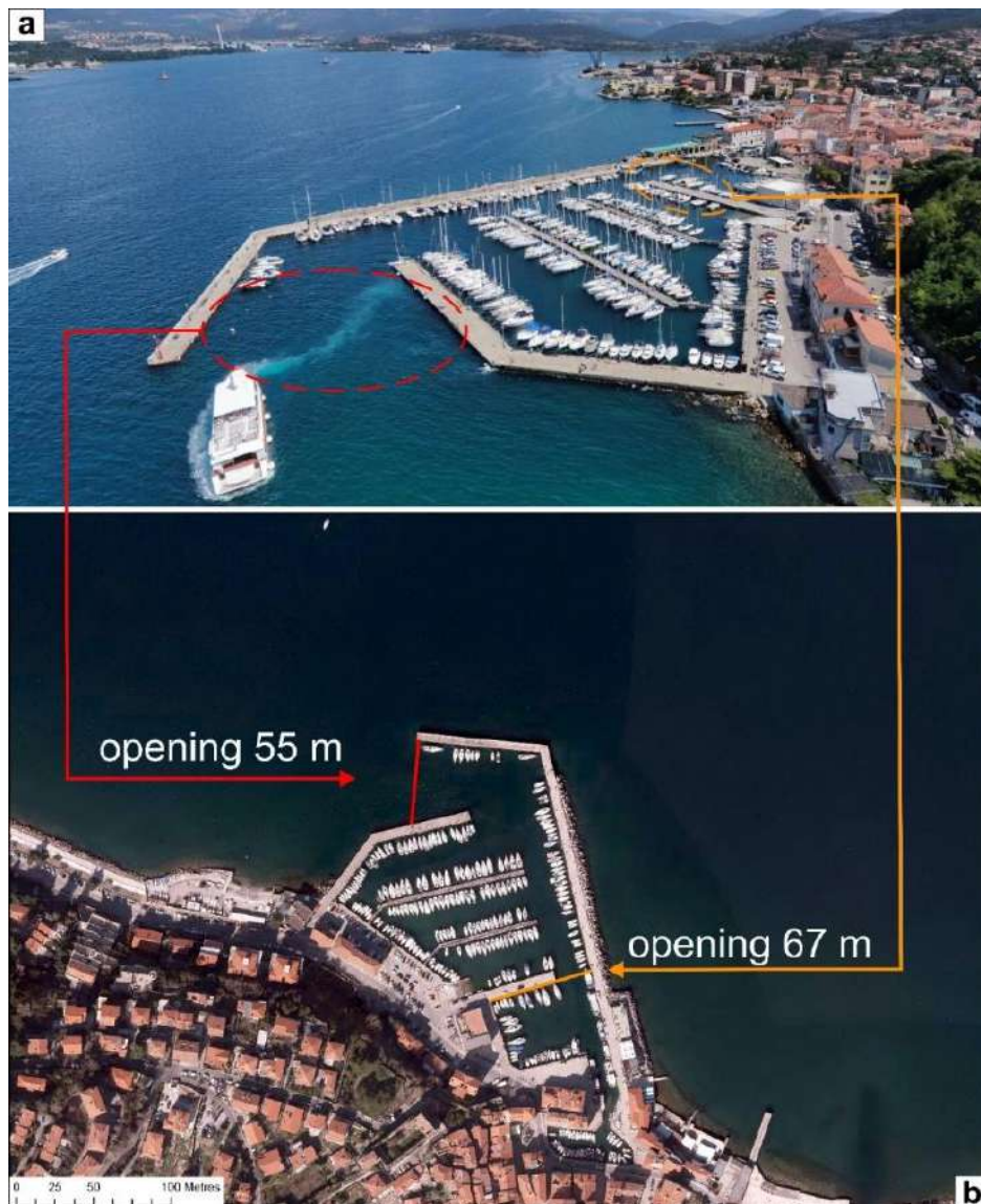
Figure 65. The Mandracchio Canal waterfront. (a) View of the Mandracchio C. marine opening (photo from Google Earth, 2025) (b) details of the different area of urban intervent to apply a movable barrier.
