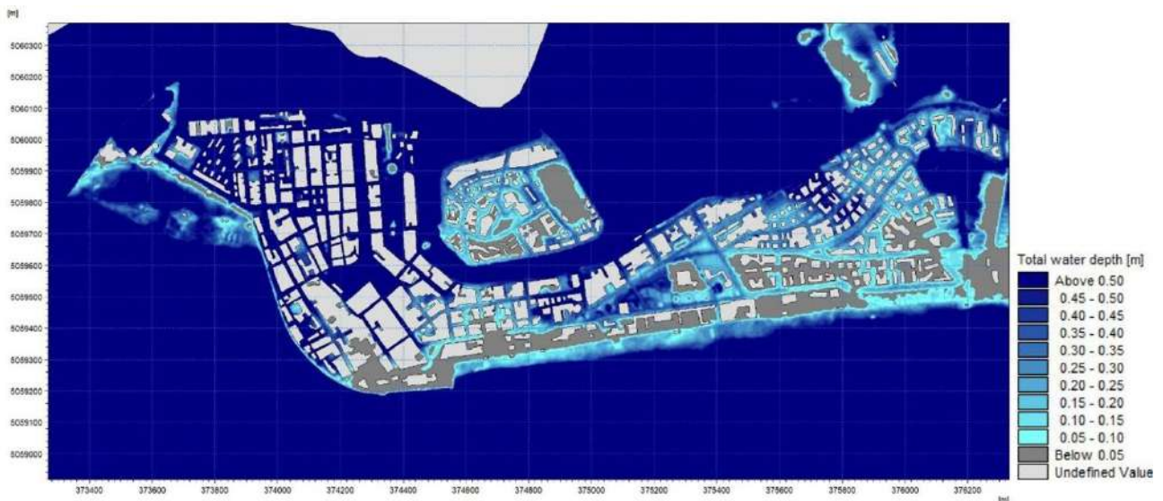
Figure 32. Maximum extent of flooding scenario for 2100, corresponding to a peak water level of 188 cm. Results obtained from a 2D hydrodynamic simulation.
