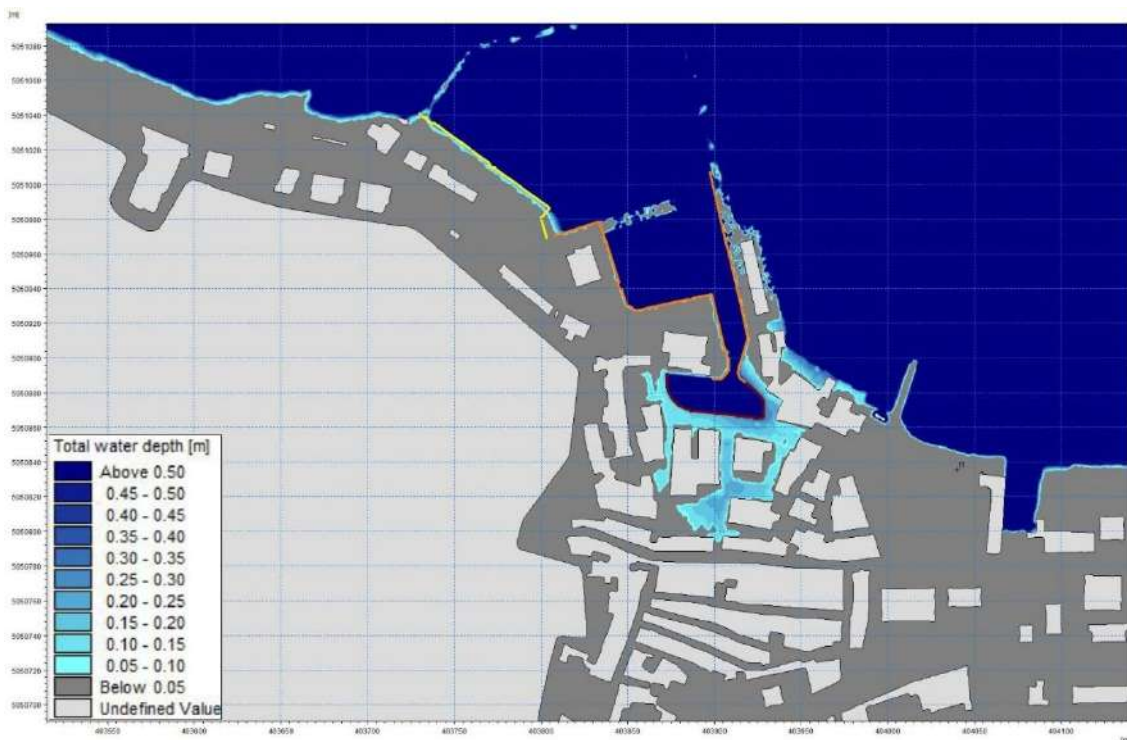
Figure 41. Maximum flood extent at a water level of 115 cm ( R_P = 2 years), obtained using the 2D HD hydrodynamic model. Water depths are limited to a maximum of 50 cm.
