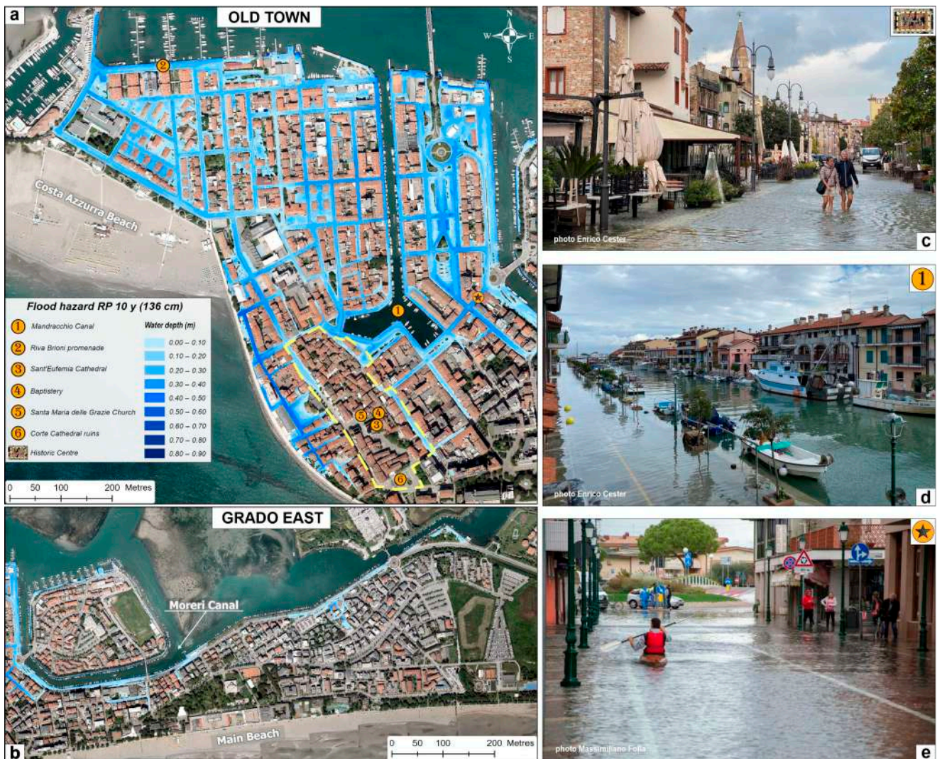
Figure 6. Flood hazard map representing an event with a 10-year RP (136 cm). The blue colours represent the water depths as a function of the city's DTM elevations: (a) The inundation map of the 'Old Town' sector shows that this area is almost entirely affected by the extent of the flooding. Flooding also affects parts of the historic centre. (b) It depicts the slight expansion of flooding to the east as well, with some ingressions of the water mass toward the built-up area by the Moreri Canal. (c) Flooding in the western part of the historic centre during 27 October 2023 (photo credits: Cester E.). (d) Expansion of the water mass along the western docks of the Mandracchio Canal during 27 October 2023 (photo credits: Cester E.). (e) expansion flooding along A. Manzoni Street during 29 October 2018 (photo credits: Folla M.).
