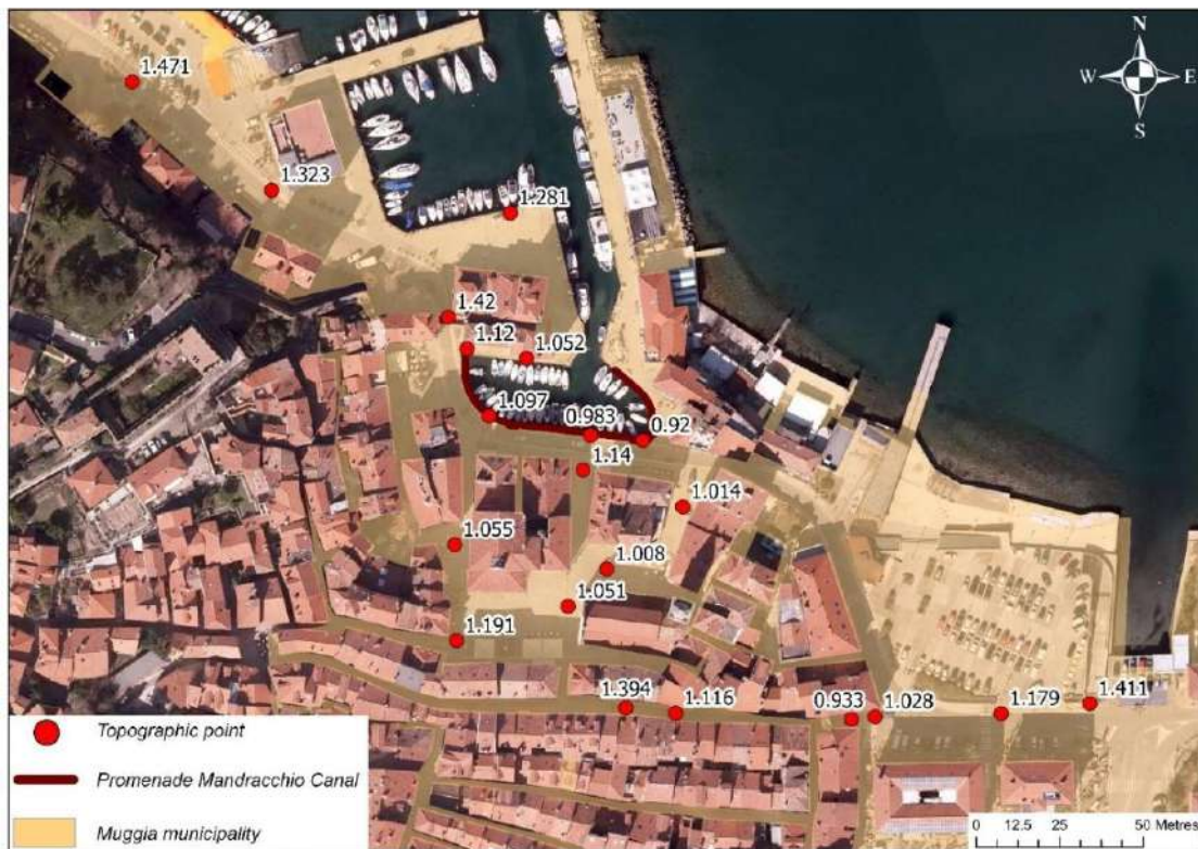
Figure 46. Topographic detail survey on historic centre area point elevation.
