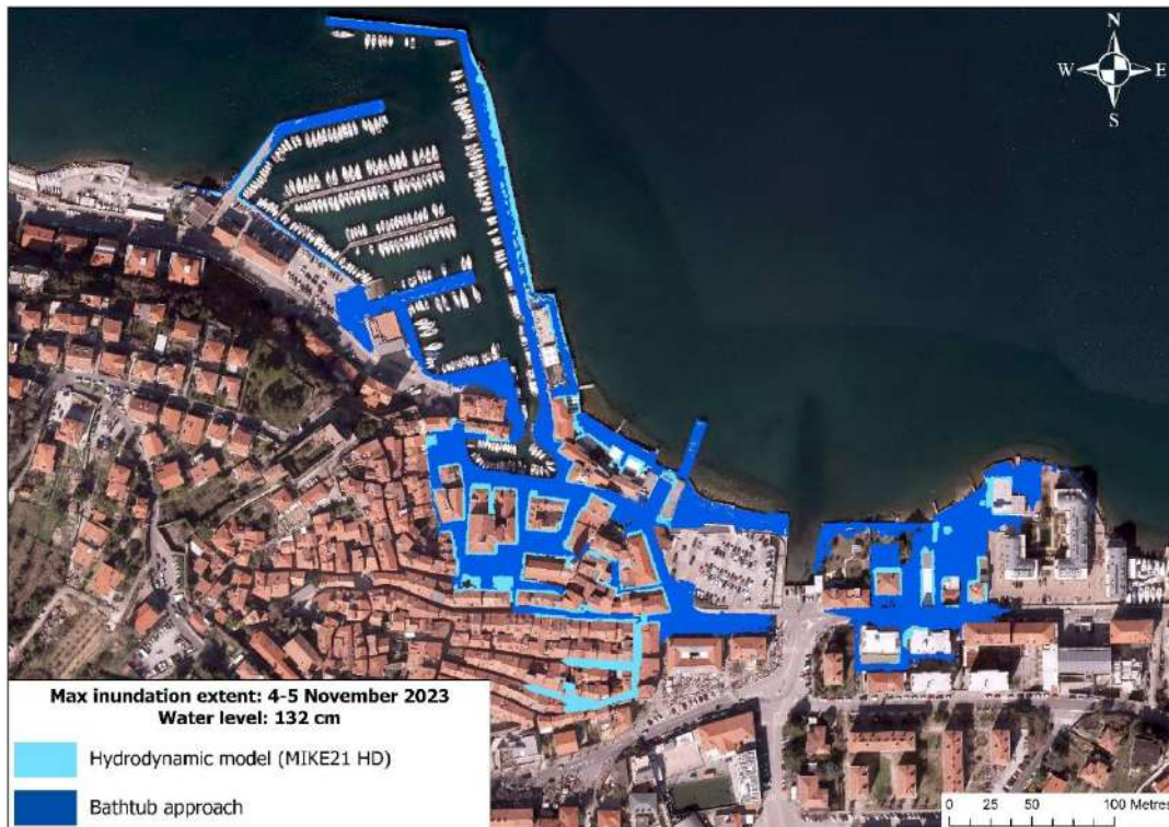
Figure 39. Maximum inundation extent for the 4-5 November 2023 event in Muggia (peak water level: 132 cm, IGM42), comparing the static bathtub approach (dark blue) and the dynamic hydrodynamic model MIKE21 HD (light blue). The dynamic simulation accounts for hydraulic constraints and flow processes, resulting in a more physically consistent flood pattern compared to the static assumption of uniform water spreading.
