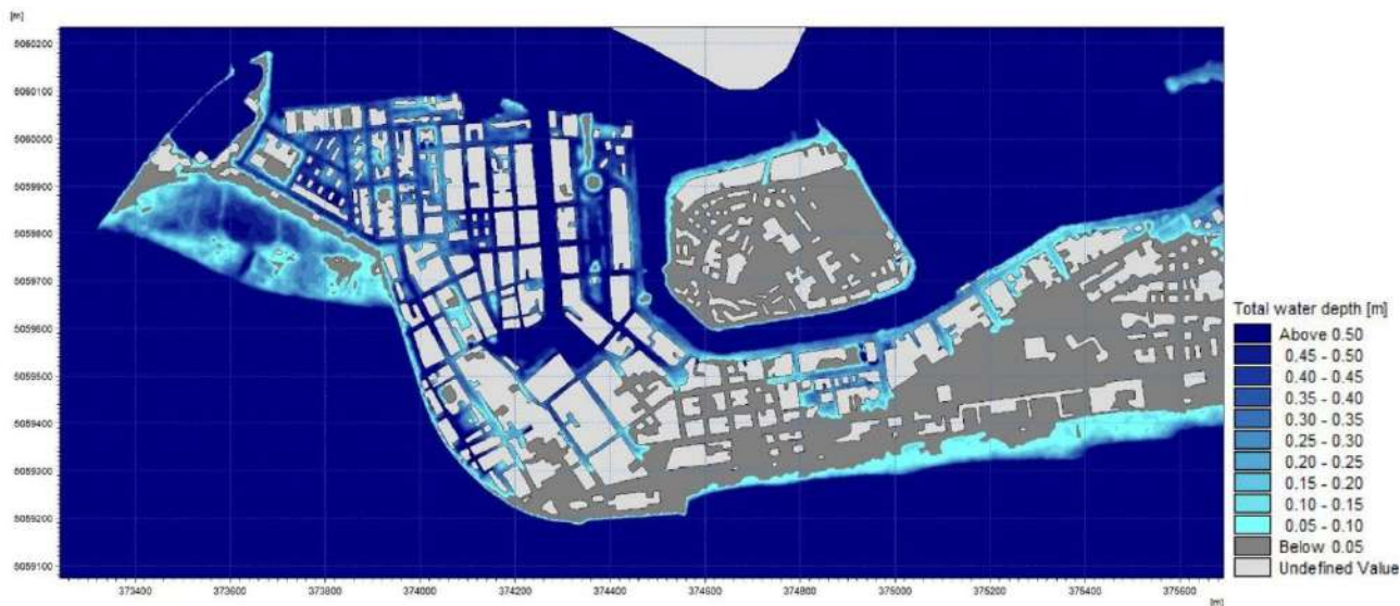
Figure 31. Maximum extent of flooding scenario for 2050, corresponding to a peak water level of 163 cm. Results derived from a 2D hydrodynamic simulation.
