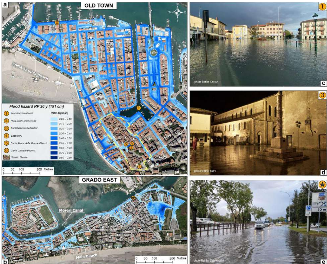
Figure 26. Flood hazard map representing an event with a 30-year R_P (151 cm). The blue colours represent the water depths as a function of the city's DTMs elevations: (a) The inundation map of the 'Old Town' sector shows that this area is completely flooded. The extent of the flooding also affects much of the historic centre. (b) The widespread flooding in the city's 'Grado East' area. Water flows inland through the Moreri Canal's embankment at several places. (c) Flooding near the southwest dock of the Mandracchio Canal during 27 October 2023 (photo credits: Cester E.). (d) Flooding in front of the St. Eufemia Cathedral during 12 November 2019 (photo credits: Patruino V.). (e) Extensive flooding along the end of the Moreri Canal embankment, Monfalcone Street during 27 October 2023 (photo credits: Rai Tgr Fvg website) (from Spadotto et al., 2025).
