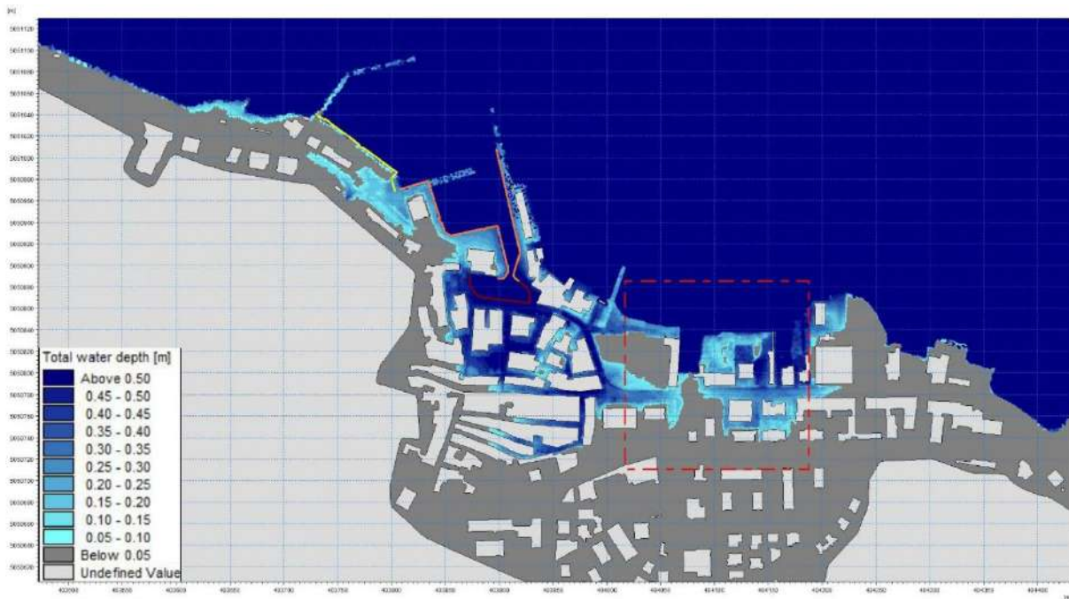
Figure 42. Maximum flood extent at a water level of 146 cm ( R_P=30 years), obtained using the 2D HD hydrodynamic model. Water depths are limited to a maximum of 50 cm.
