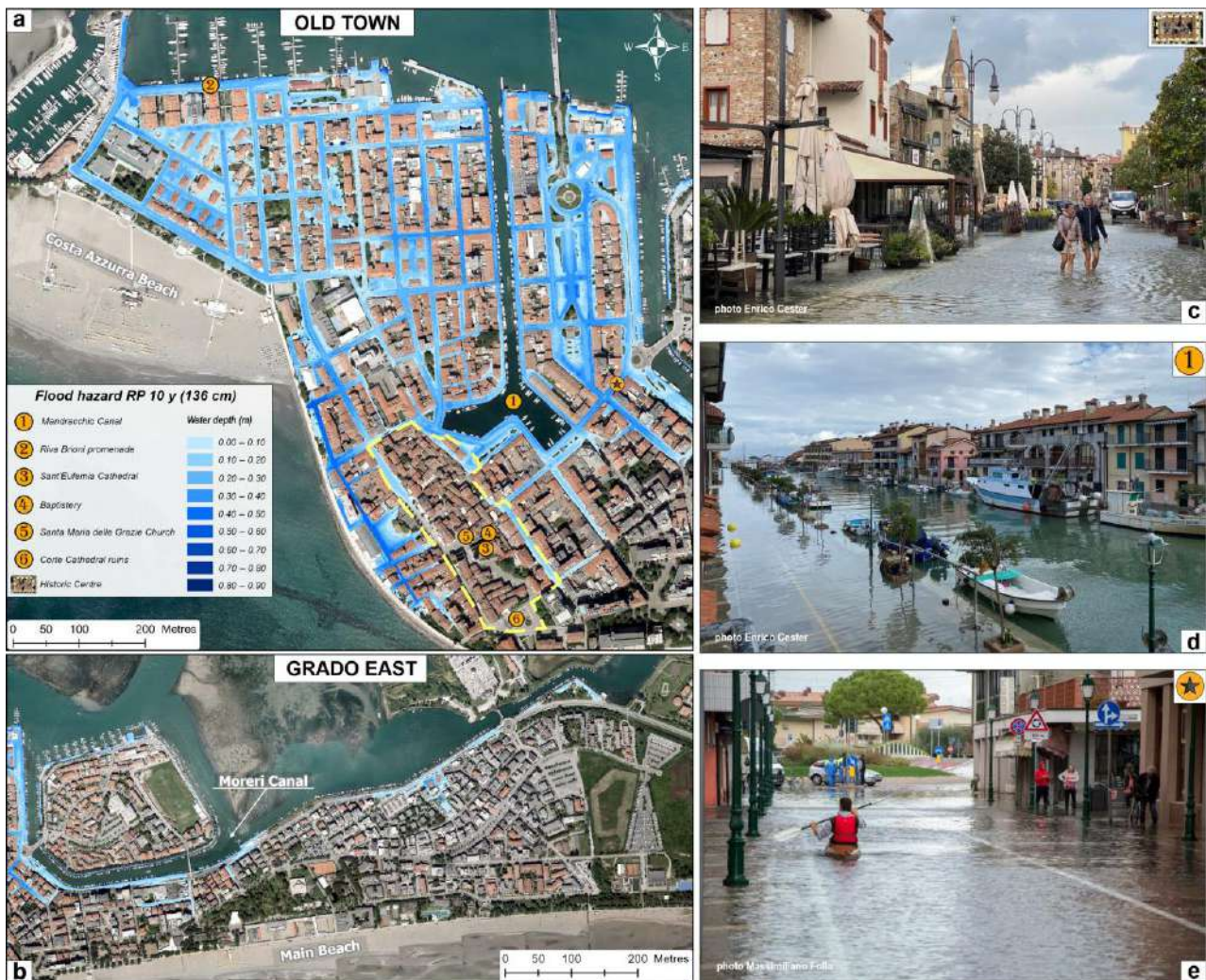
Figure 25. Flood hazard map representing an event with a 10-year R_P (136 cm). The blue colours represent the water depths as a function of the city's DTM elevations: (a) The inundation map of the 'Old Town' sector shows that this area is almost entirely affected by the extent of the flooding. Flooding also affects parts of the historic centre. (b) It depicts the slight expansion of flooding to the east as well, with some ingressions of the water mass toward the built-up area by the Moreri Canal. (c) Flooding in the western part of the historic centre during 27 October 2023 (photo credits: Cester E.). (d) Expansion of the water mass along the western docks of the Mandracchio Canal during 27 October 2023 (photo credits: Cester E.). (e) expansion flooding along A. Manzoni Street during 29 October 2018 (photo credits: Folla M.) (from Spadotto et al., 2025).
