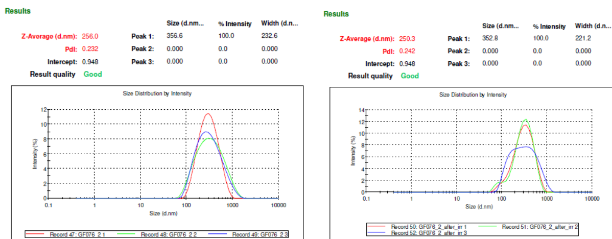
Figure S60. DLS measurement of AL3 before (left) and after (right) 3h irradiation. Before: Z-average 256.0 nm, PDI = 0.232; after: Z-average 250.3 nm, PDI = 0.242.
