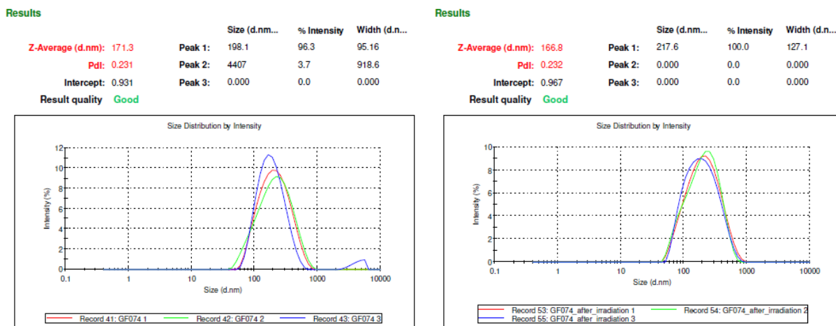
Figure S59. DLS measurement of AL1 before (left) and after (right) 3h irradiation. Before: Z-average 171.3 nm, PDI = 0.231; after: Z-average 166.8 nm, PDI = 0.232.
