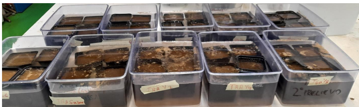
Figure 1. Fresh soils (OF and CF) immersed with fresh or saline waters for 6 h.
