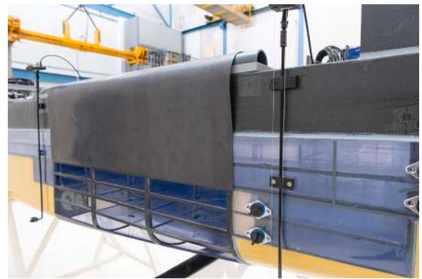
Fig. 7. Breach opening and the magnetic cover (photo courtesy of MARIN).
