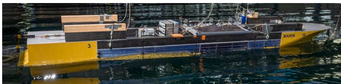
Fig. 14. Cruise ship model in irregular beam seas (courtesy of MARIN).
