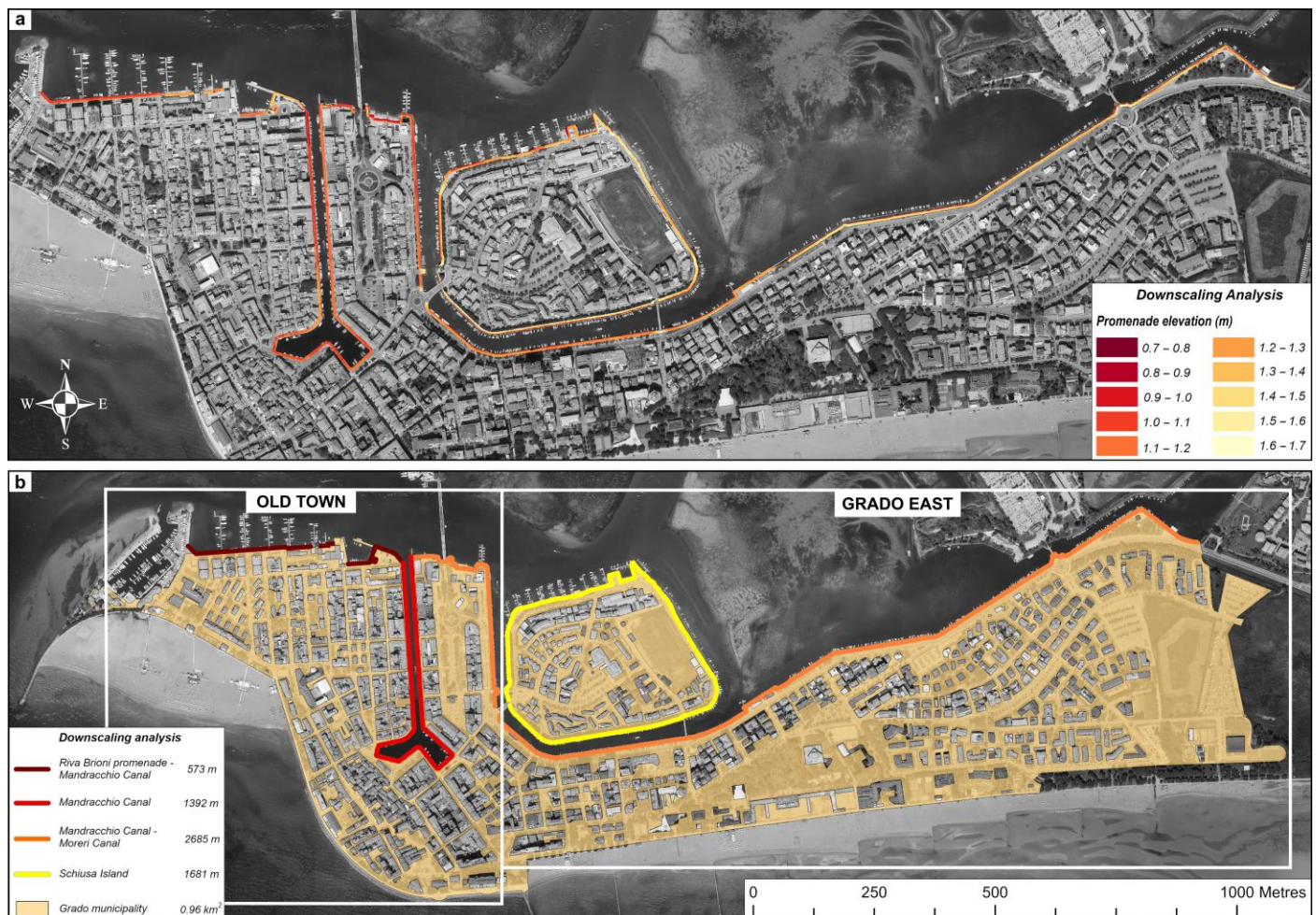
Figure 2. Downscaling area analysis: (a) elevation of the lagoon promenade considered in the study, represented by 10 classes subdivided every 0.10 m of elevation. (b) The subdivision of the promenade and lagoon embankment into 4 macro sectors; the extent of the inhabited area of Grado municipality is also reported, treating the streets as unobstructed surfaces for water flow while omitting buildings and uninhabited areas.
