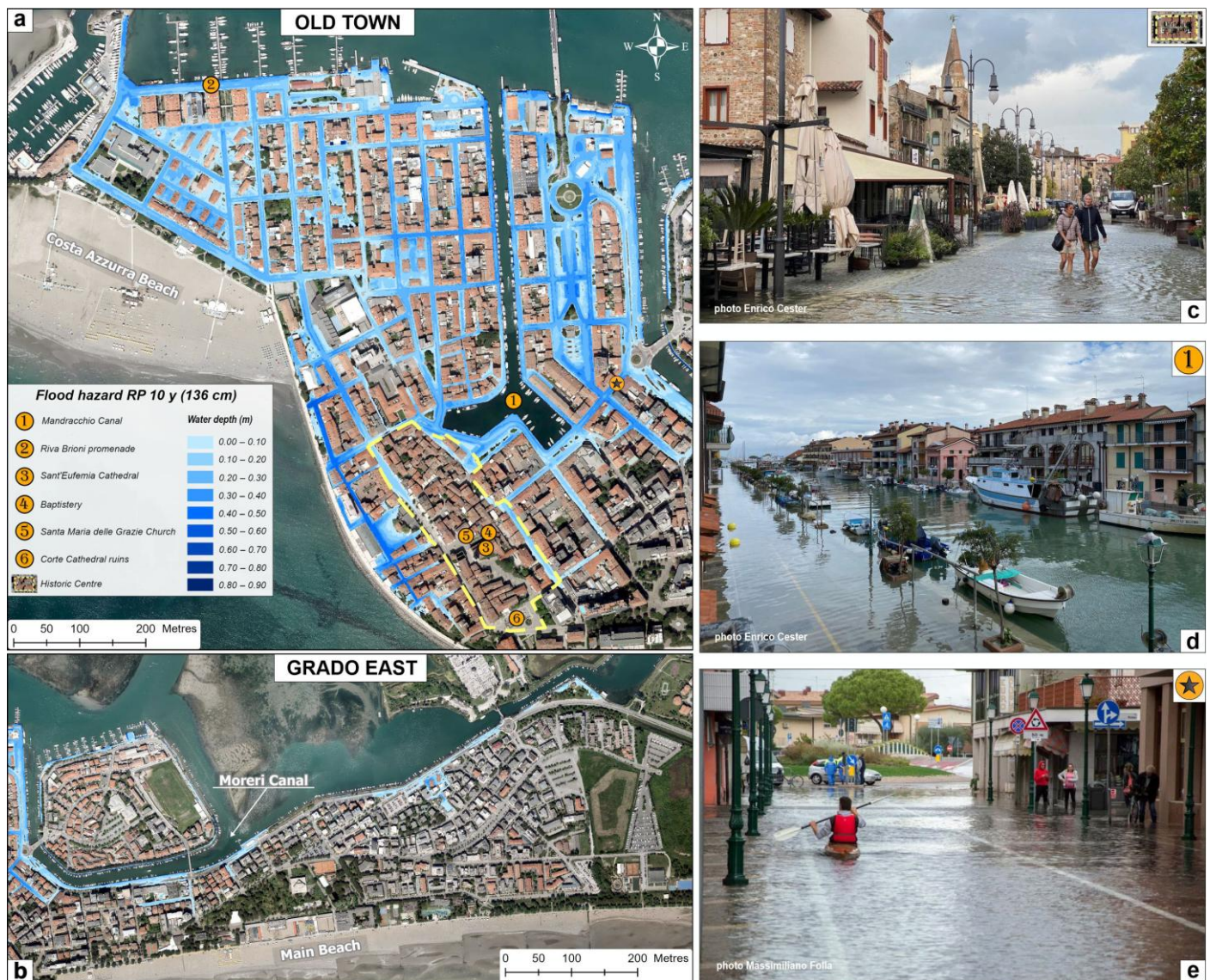
Figure 6. Flood hazard map representing an event with a 10-year RP (136 cm). The blue colours represent the water depths as a function of the city's DTM elevations: (a) The inundation map of the 'Old Town' sector shows that this area is almost entirely affected by the extent of the flooding. Flooding also affects parts of the historic centre. (b) It depicts the slight expansion of flooding to the east as well, with some ingressions of the water mass toward the built-up area by the Mureri Canal. (c) Flooding in the western part of the historic centre during 27 October 2023 (photo credits: Cester E.). (d) Expansion of the water mass along the western docks of the Mandracchio Canal during 27 October 2023 (photo credits: Cester E.). (e) expansion flooding along A. Manzoni Street during 29 October 2018 (photo credits: Folla M.).
