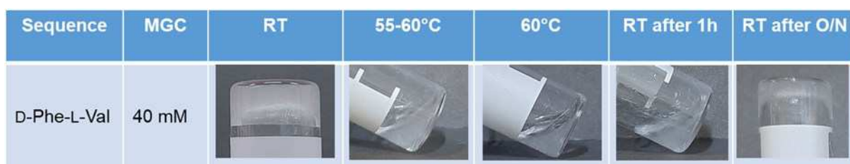
Figure 7.18. Thermoreversibility test for D-Phe-L-Val hydrogel with a melting temperature between 55-60 °C. Reproduced from Ref. [1] with permission from © 2022 Royal Society of Chemistry.
