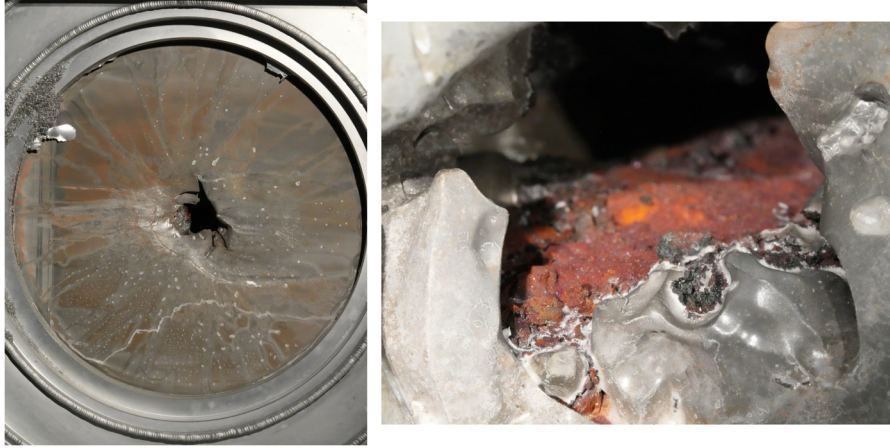
Figure A.1: Pictures of the cavity discovered in the second-generation n_TOF spallation target. Pictures from O. Aberle.
