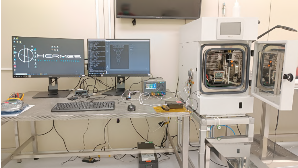
Figure 4.9: The calibration experimental setup. The payload is in the climatic chamber, on the right [106].
