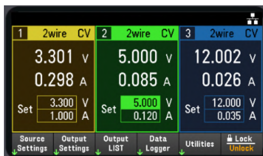
Figure 4.15: The three low-tension supplies (3.3 V, 5 V, 12 V) with the associated current absorptions (298 mA, 85 mA, 26 mA) shown on the low voltage generator screen during preliminary tests.
