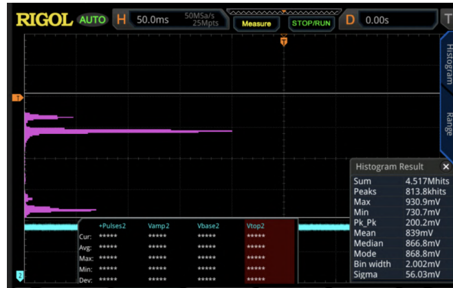
Figure 4.7: Example of a single-channel spectrum recorded by the oscilloscope in purple. The three emission lines are clearly visible: one from ^{55}\text{Fe} at 5.9 keV, and two from ^{109}\text{Cd} at 22.1 keV and 24.9 keV.
