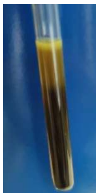
Figure 2.20. NMR tube of the mixture of 1b + MA + E in TFE- d_3 after one week at room temperature: the precipitated copolymer is evident.
