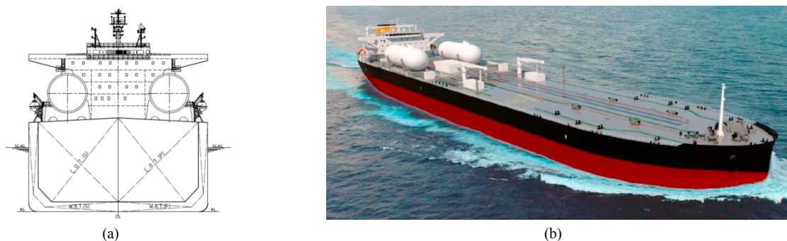
Fig. 4. Arrangement of the LNG C-Type tanks as seen from a transversal section (a) and in a rendering (b).
