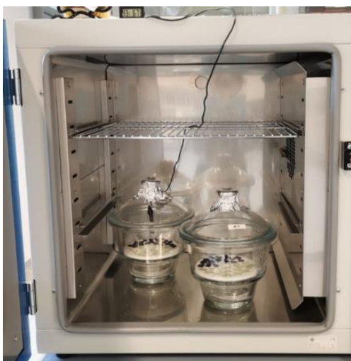
Figure 6.2. Set-up for the experimental ageing of glass mock-ups.
