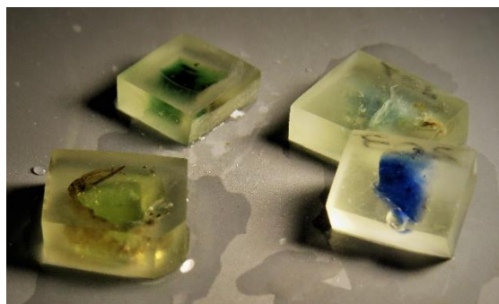
Figure 2.2. Small pieces of the glass samples embedded in epoxy resin and polished for LA-ICP-MS analyses.
