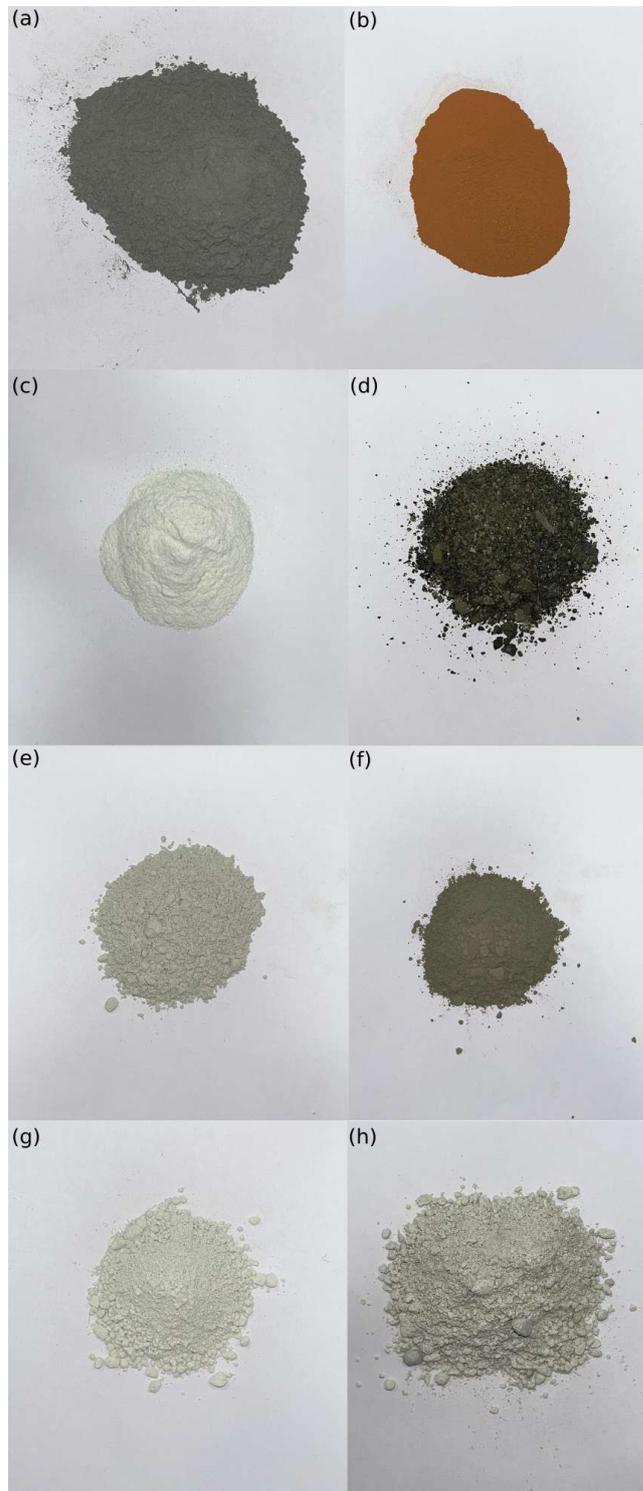
Figura 8.2: Esempi di RHA (a), BD (b), MD (c), SD (d), FA (e), OPC (f), LD (g) e SF (h).
