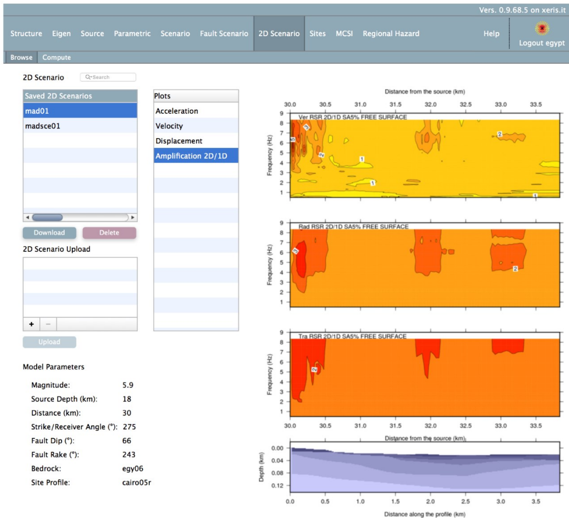
Figure 9 Amplifications (dark red areas) are shown with respect to a laterally homogeneous bedrock model for the “Madrasa” profile. From top to bottom, the amplifications are shown along the profile for the vertical, radial, and transverse components. The abscissa shows the position along the profile, represented at the bottom, while the ordinates in the upper images refer to the frequencies at which the amplifications eventually occur.
