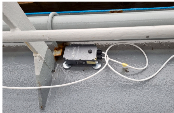
Fig. 2. (a) Sensor positions and (b) Dewesoft IOLITE mems triaxial accelerometer.
