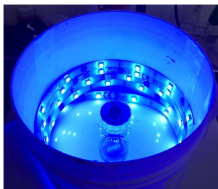
Figure SI.EP-23. LEDs tape irradiation experiment
