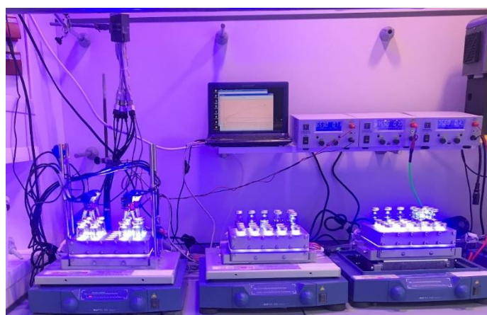
Figure SI.EP.EP-2. In-house developed parallel photoreactors.
