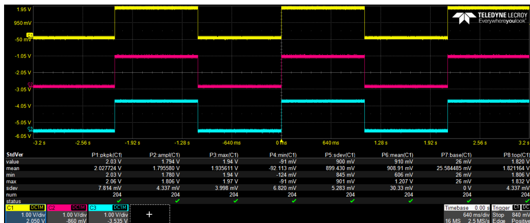
Figure 9. PPS signal after PTP implementation.
