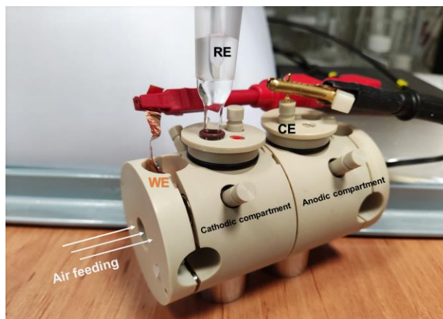
Figure S28. Experimental set-up employed for bulk electrolysis with an air gas diffusion electrode in the cathode compartment. The electrochemical cell is in H-cell configuration with two different compartments separated by Nafion 117 membrane. Particularly, air was let feeding spontaneously from one side of the working electrode (WE) and the other side was in contact with aqueous electrolyte. Ag/AgCl was the reference electrode (RE). Pt wire was used as the counter electrode (CE) is in the other chamber.
