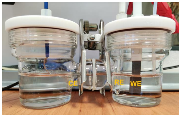
Figure S19. Experimental set-up employed for bulk electrolysis with planar electrodes. The electrochemical H-cell features two different compartments separated by a Nafion 117 membrane. Working electrode (WE) and Ag/AgCl reference electrode (RE) are in one chamber. Pt foil as the counter electrode (CE) is placed in the other chamber.
