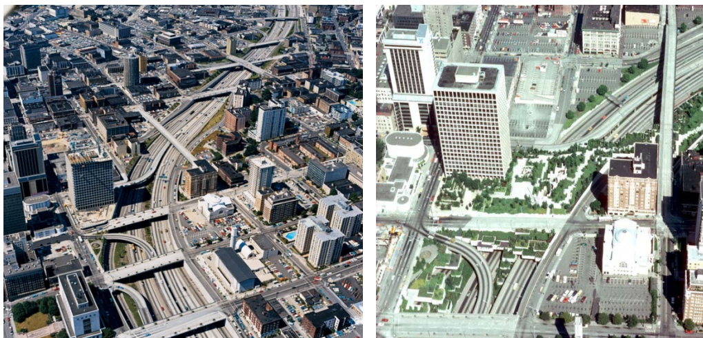
Figure 5. On the Left: Interstate 5 before the Highway Lid and Freeway Park. On The Right: Highway Lid and Freeway Park
