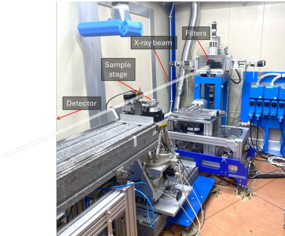
FIGURE 4.16: Photograph of the beamline's experimental hutch. The detector is not shown as it is placed downstream.
