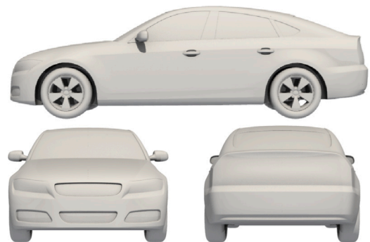
Fig. 4. DrivAer in fastback configuration: on top — side view; on bottom from left to right — front and back views.
