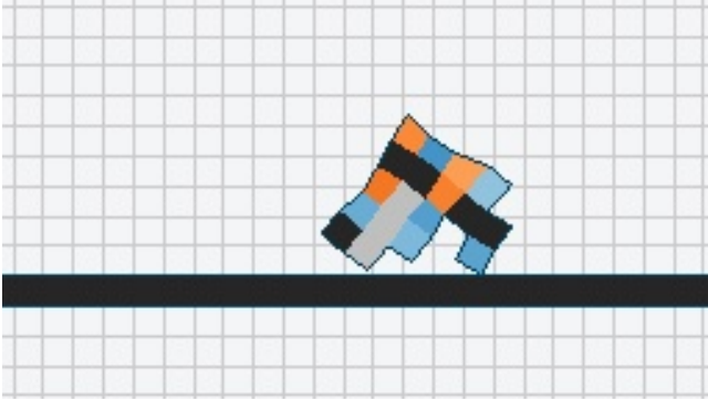
Figure 2: A voxel-based soft agent. The voxel color stands for the material: black is rigid inactive, gray is soft inactive, orange is a horizontal actuator, and cyan is a vertical actuator.
