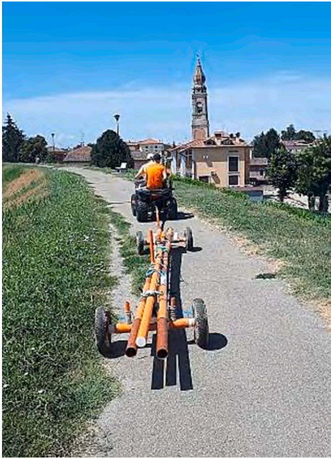
Fig. 4. Acquisition phase during the dry survey. The CMD-Explorer by GF Instruments has been mounted on a PVC and Teflon sledge and towed by a quad to cover 60 km of levees (performed two times, one for each coil's configuration – HIGH and LOW, for a total of 120 km).
