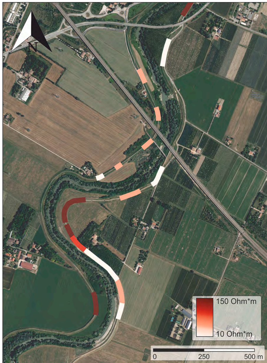
Fig. 8. An example of the results obtained from the difference between dry and wet FDEM surveys shows resistivity differences plotted along the levees, providing a zonation of areas prone to higher vulnerability.
