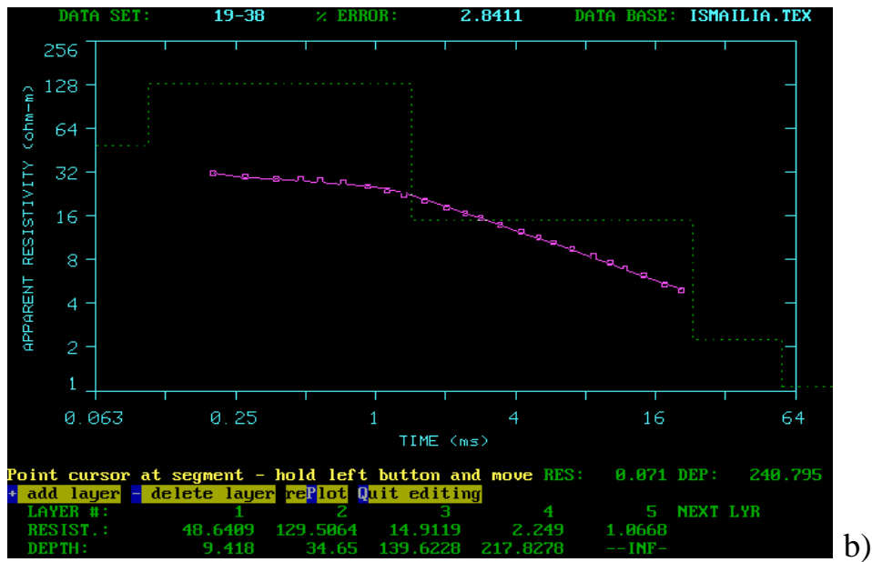
Fig. 4. 6: Exemplary multi-layer model obtained from TEM data inversion at station No. 3 (a) and 19 (b).
