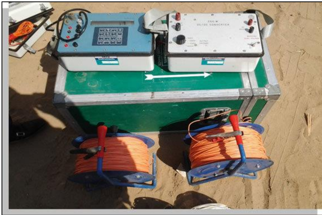
Fig. 3. 7: SYSCAL R2 resistivity meter and its components.
