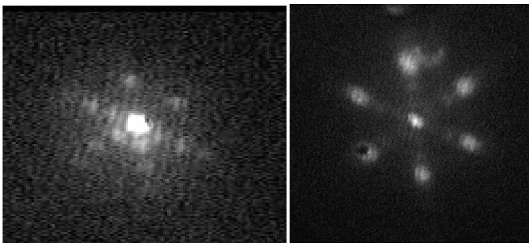
Figure S3. LEED diagrams at different coverages showing the extra spots observed close to the reconstruction ones.
