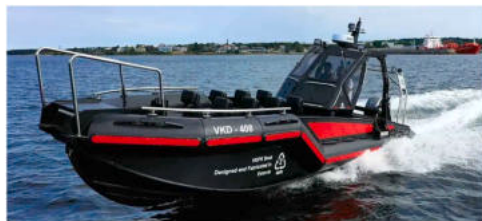
Fig. 1. HDPE workboat ( https://workboat365.com/wp-content/uploads/2023/11/6.webp ).
