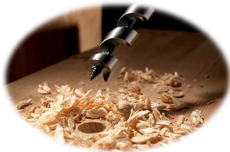
Figure 7: Wood drilling with a cemented carbide tool.
