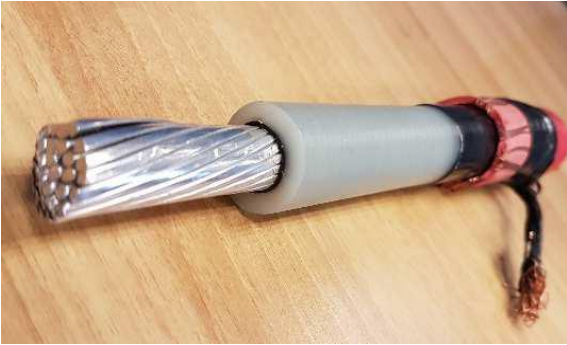
Fig.2. Example of XLPE insulated MV cable used in the PD tests.
