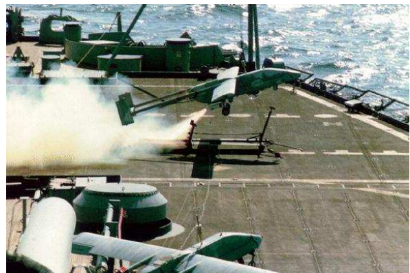
Figure 1 RATO launching a UAV (source: https://www.globalsecurity.org/intell/systems )
