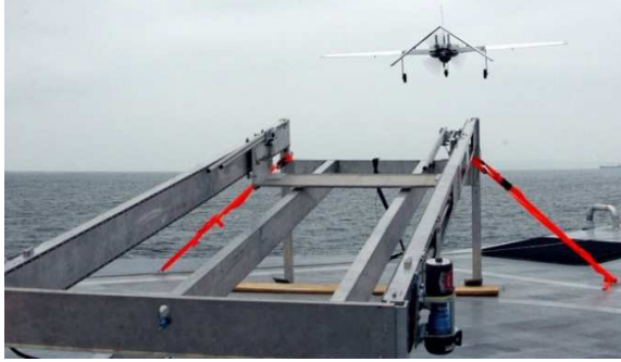
Figure 2 UAV take-off from a bungee cord launcher from navy.mil
