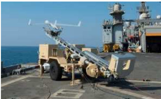
Figure 3 Hydraulic catapult launching a UAV (source: malaysiandefence.com)
