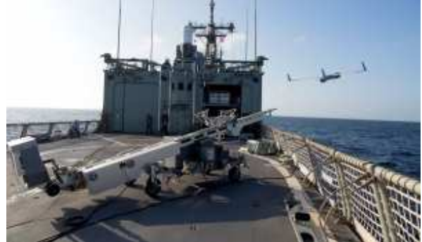
Figure 4 Scan Eagle UAV launch by a pneumatic catapult (source: navy.gov.au)
