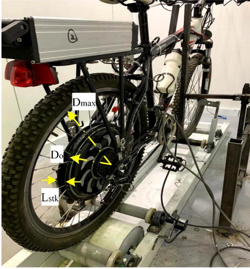
Fig. 4. Commercial BLDCM mounted on an e-bike in the lab with relevant dimensional constraints.
