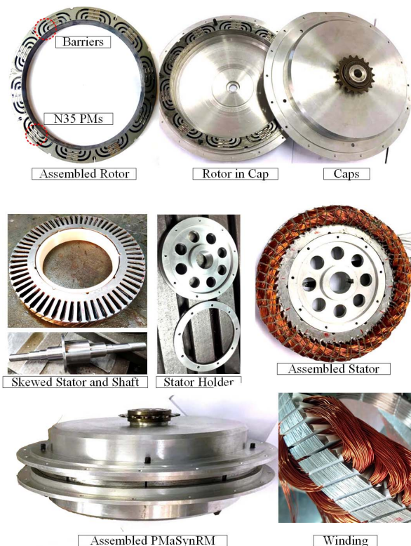
Fig. 9. Different parts of the prototyped PMaSynRM.
