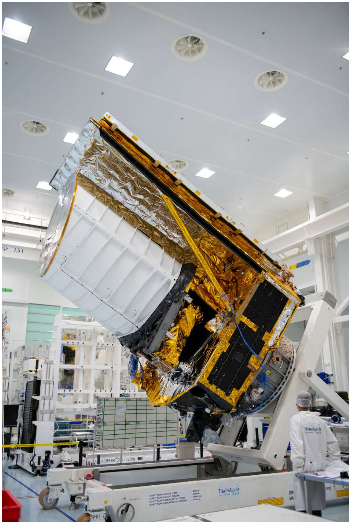
Figure 2.1: Structural and thermal model of the Euclid satellite. Picture taken from https://sci.esa.int/web/euclid/multimedia-gallery .
