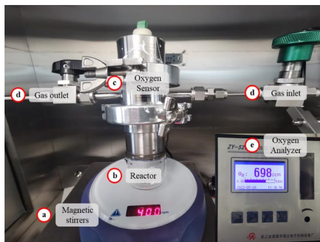
Figure S9. Image of the in-situ oxygen consumption analyzing system. The reactor (b) is placed on the magnetic stirrer (a) and combined with an oxygen sensor (c) and gas line (d). The oxygen analyzer (e) is connected with the oxygen sensor (c).
