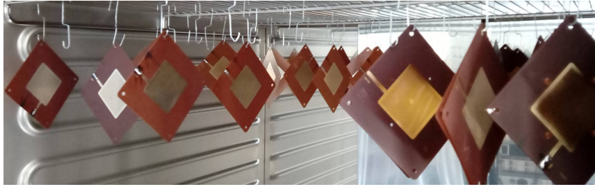
FIGURE 9.6: The produced THGEMs drying in the oven.
