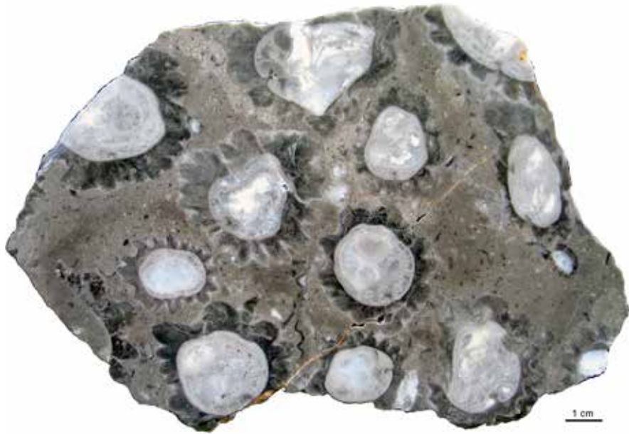
Figure 3.3.11: Polished slab of Lipica Limestone displaying a cross-section of rudist cluster (Photo: Bogdan Jurkovšek)
