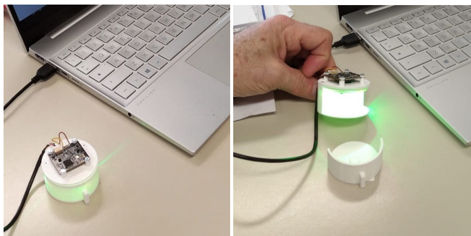
Figure 3.46- Image reader in-lab built device.
