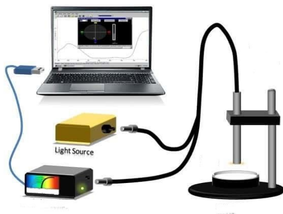
Figure 3.44 -General scheme of the optical fiber spectrometer. 25
