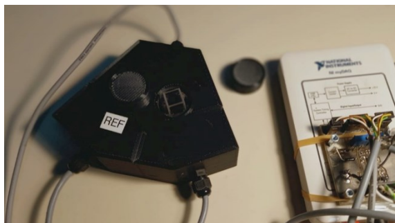
Figure 3.16- In-lab built photometer to perform analysis in cuvette.
